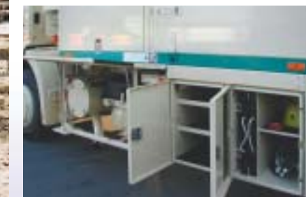
A 3-axle chassis allows special-purpose magazines and storage compartments to be attached
