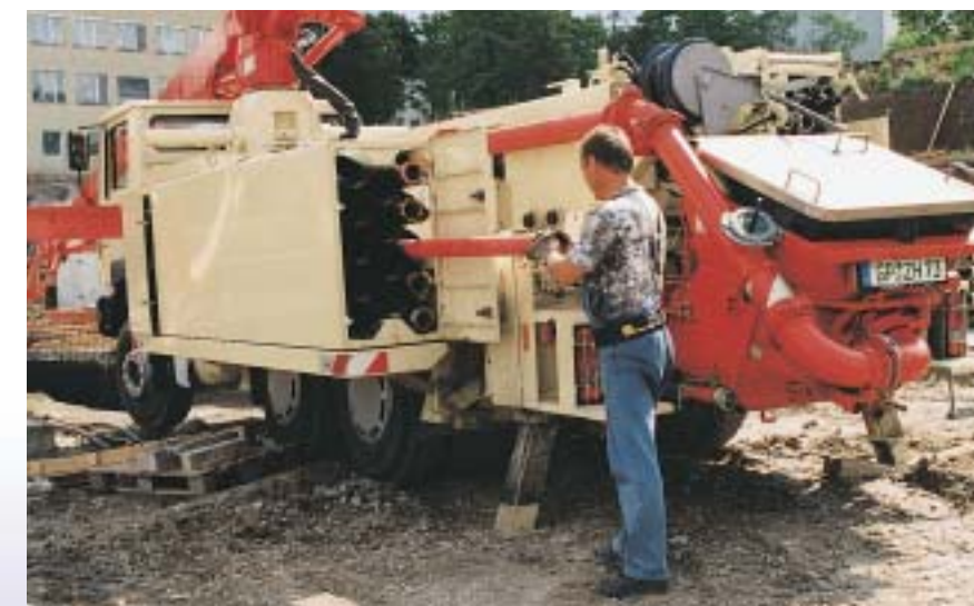
Loading and unloading of pipes and hoses is very simple using a hydraulically-lowered container
